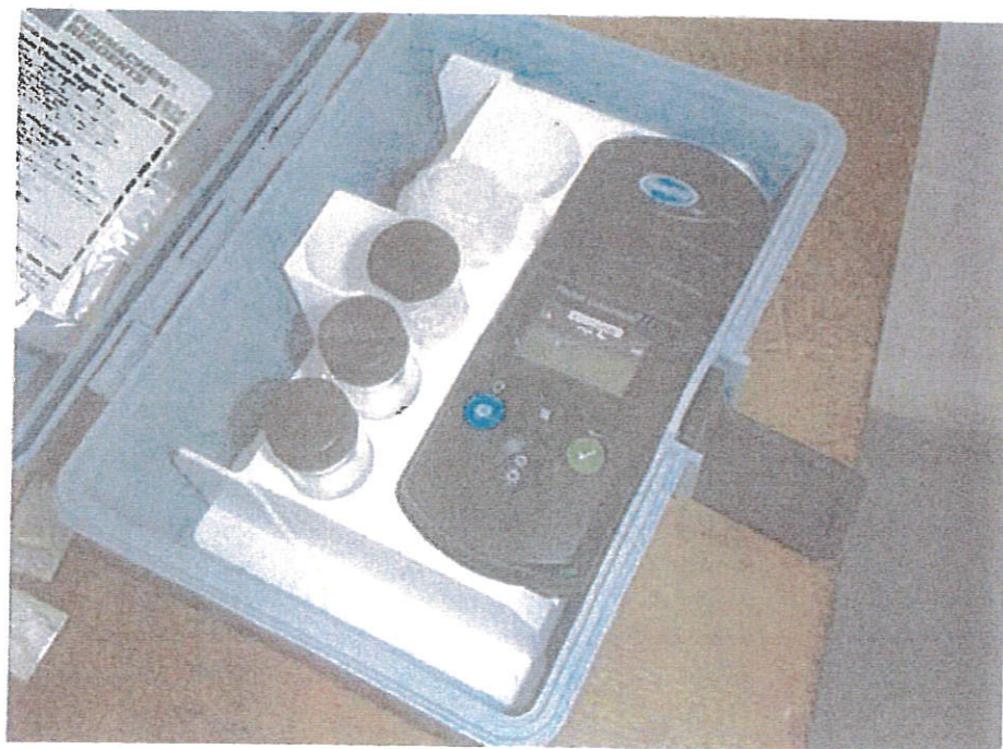
Louisville East POTW; Hach chlorine test kit
